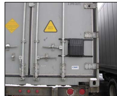
GlobalEyes+ Wedge – Integrated Electronics and Antenna (Remote Sensor Node required for internal sensors)
